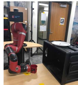
(a) In the pouring task, the robot must pick a cup off of the table and pour its contents into a bowl without spilling.
